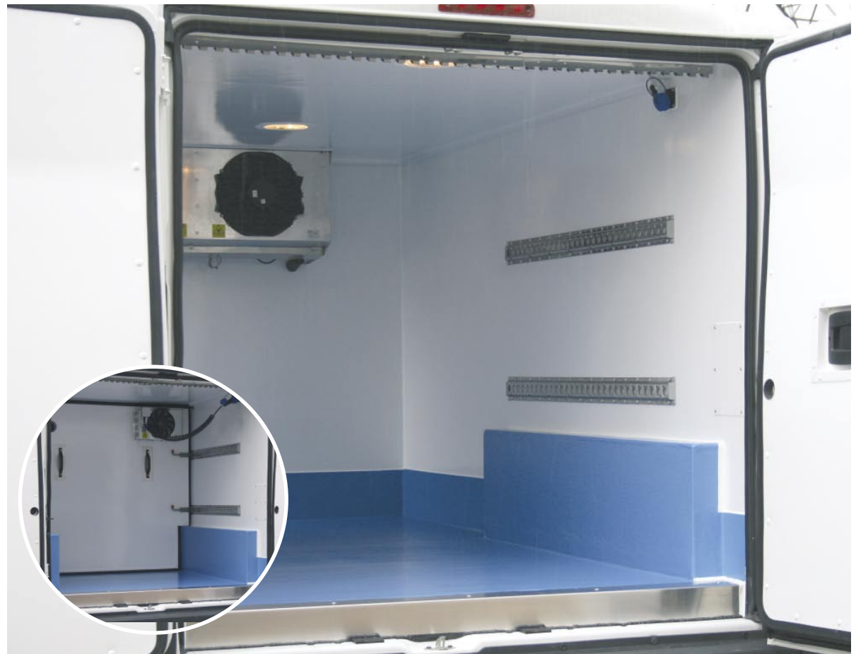
Removable bulkhead allows variable sizing of two temperature zones, or just one zone when your load mix changes
