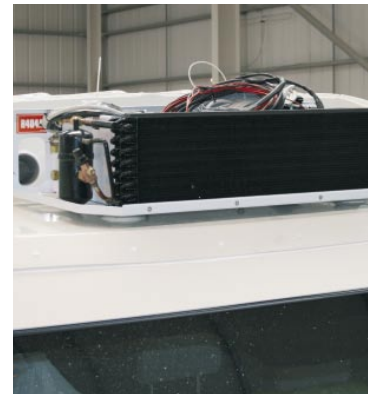
Condenser unit being fitted into recessed GRP housing
